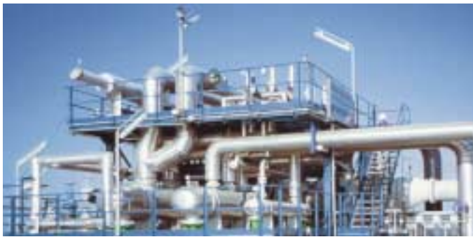
Vacuum unit for an MSF sea water desalination plant
