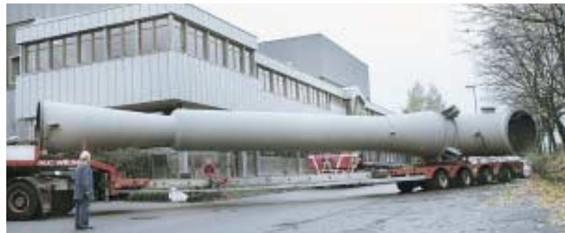
Jet pump for a 4-stage jet vacuum pump for steel degassing suction flow: 1,100 kg/h or 1,387,000 m 3 /h, suction pressure abs.: 0.6 mbar
