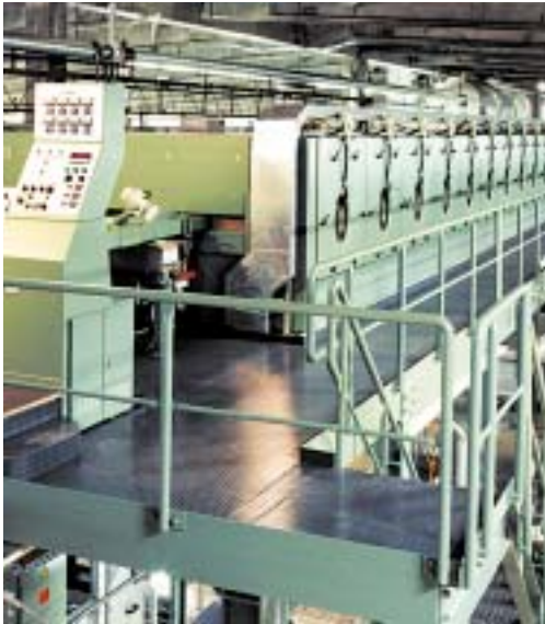
Top left: Plant for the drying of chemicals equipped with stainless steel heat exchangers
