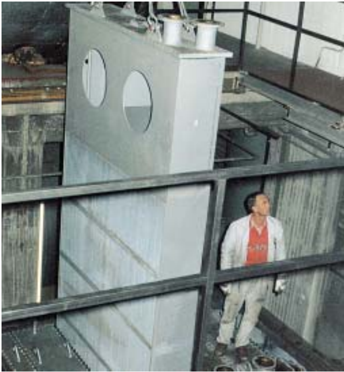
Top left: Plant for the drying of chemicals equipped with stainless steel heat exchangers
